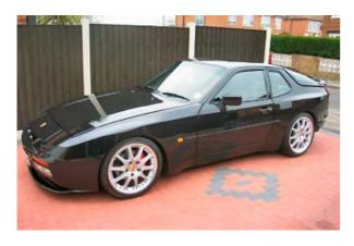
Notice the twin vent badge panel – this was custom made to channel more air into the intercooler located beneath. The car also benefits from a sensational set of 18" split rim alloy wheels and has recently also been the subject of the monobloc front calliper upgrade – more details on this next month! A custom front air splitter completes the purposeful look of this great looking car. So what's under the bonnet?
