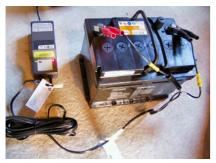
battery will drained to the point where it will no longer have the capacity to start the car. Its well worth using а battery conditioner and charging system such as the Carcoon system shown
